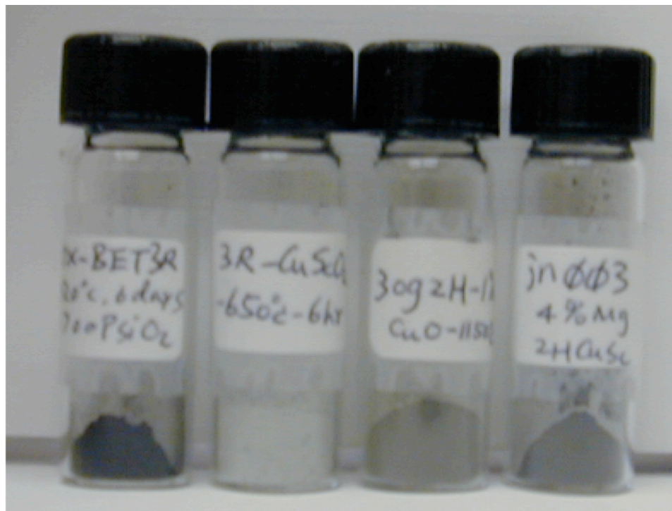
Fig.3.18. Powder colors of the intercalated 3R \text{CuScO}_2 (left), unoxidized 3R and 2H polytypes, and 4 at. % Mg doped.
