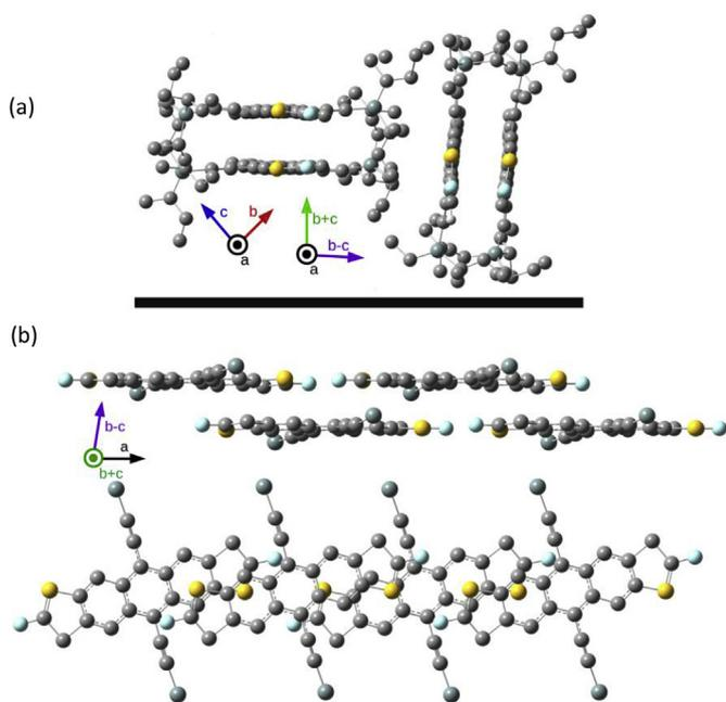
**Fig. 3.** Molecular packing of the diF TSBS-ADT derivative. (a) Side view; black line corresponds to the substrate. The substrate coincides with the (011) crystal orientation. (b) Top view of the plane in which the charge transport is measured in our experiments. Side groups are cropped for clarity. Crystal axes are also shown.
