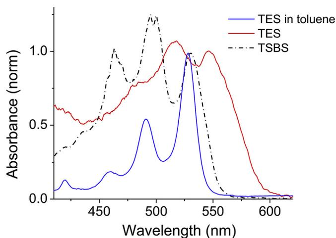
**Fig. 4.** Optical absorption spectra of representative diF TES-ADT and diF TSBS-ADT crystals. Optical absorption from a dilute solution of diF TES-ADT (identical to that of diF TSBS-ADT) in toluene is also shown.
