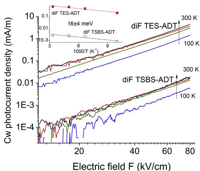
Fig. 9. Photocurrent densities obtained under 532 nm 2 mW/cm $^2$  cw excitation as a function of applied electric field at various temperatures in diF TES-ADT and diF TSBS-ADT crystals. Inset shows temperature dependence of photocurrent densities measured at 40 kV/cm in both types of crystals. Arrhenius fits and activation energies are also included.
