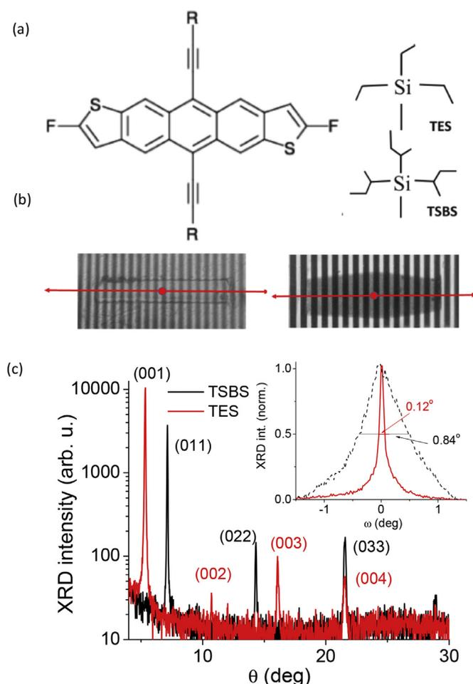
**Fig. 1.** (a) ADT derivatives under study. (b) Images of solution-grown ADT crystals on interdigitated electrodes (vertical lines) spaced by 25  $\mu\text{m}$ . Red line corresponds to a “long crystal axis” and the direction of applied electric field. (c) XRD data on representative diF TES-ADT and diF TSBS-ADT crystals. Inset shows rocking curves. (For interpretation of the references to colour in this figure legend, the reader is referred to the Web version of this article.)
