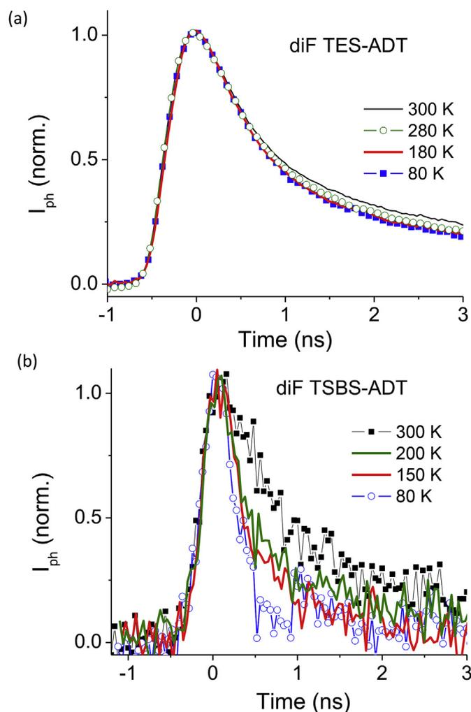
**Fig. 8.** Normalized photocurrents at various temperatures in (a) diF TES-ADT and (b) diF TSBS-ADT crystals.
