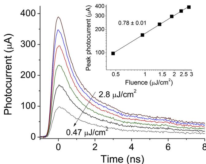
Fig. 6. Time-resolved photocurrent in diF TES-ADT at 300 K at various excitation pulse fluences (2.8  $\mu\text{J}/\text{cm}^2$ , 2.4  $\mu\text{J}/\text{cm}^2$ , 1.9  $\mu\text{J}/\text{cm}^2$ , 1.4  $\mu\text{J}/\text{cm}^2$ , 0.94  $\mu\text{J}/\text{cm}^2$ , and 0.47  $\mu\text{J}/\text{cm}^2$ ). Inset shows photocurrent peak dependence on the fluence.
