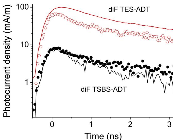
Fig. 5. Time-resolved photocurrent density obtained under 532 nm pulsed excitation at the pulse fluence of 1.2  $\mu\text{J}/\text{cm}^2$  and applied electric field of 40  $\text{kV}/\text{cm}$  at 300 K.
