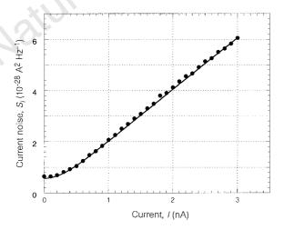
**Figure 2** Quantum shot noise as a function of direct current, l, through the QPC without an applied magnetic field (circles). The solid line is equation (2) with the temperature (57 mK) deduced from Fig. 1. The transmission, t, is 0.37.
