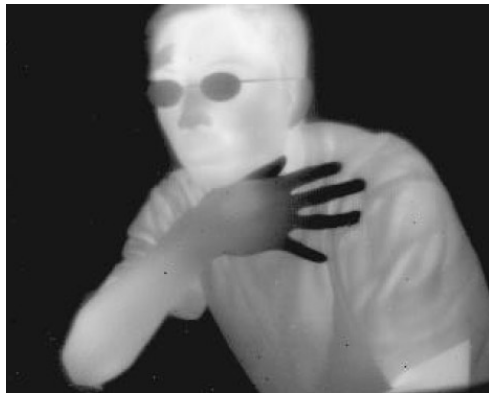
MWIR InGaAs/InAlAs/InP QWIP 320x256 FPA camera (at 100 K)
