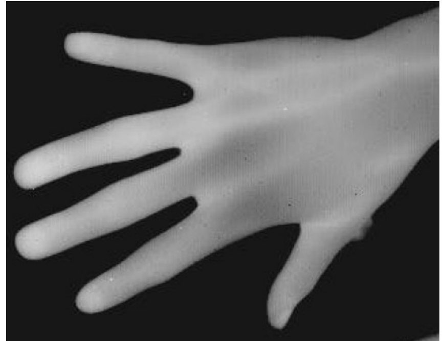
MWIR InGaAs/InAlAs/InP QWIP 320x256 FPA camera (at 100 K)
