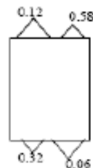
Four silicon nitride cantilevers showing constants (N/m)
