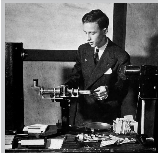
Taken at December 1940 Science Congress talk. At left is a 6 inch richest-field telescope f4, much more portable than my original f8, in the center is the diffraction grating spectroscope, at right a photomicrographic camera, with odd bits of paraphernalia in the foreground.
