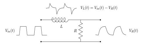
(a) Repeat the same measurements for the LR circuit.
