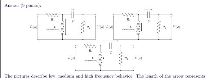
The pictures describe low, medium and high frequency behavior. The length of the arrow represents the amplitude of the current.
