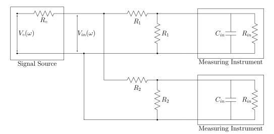
(a) When  $\omega = 10^5$  Hz, will  $Z_{in}(\omega)$  for the oscilloscope significantly effect the measured output of either divider?
