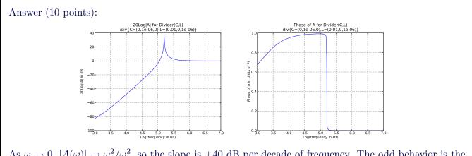
As  $\omega \to 0$ ,  $|A(\omega)| \to \omega^2/\omega_{\circ}^2$ , so the slope is +40 dB per decade of frequency. The odd behavior is the peak at  $\omega_{\circ}$ , with  $|A(\omega)| = 10^4$ . This happens because, for this nearly-undamped resonantor, energy is continually added to the oscillator. A finite resistance  $r = 0.01 \ \Omega$  was required to keep the amplitude finite at  $\omega_{\circ}$ .
