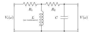
(a) Consider the circuit to be two consecutive filters with transmission functions  $A_1(\omega)$  and  $A_2(\omega)$ . Use physical reasoning and the concept of impedance to explain thoroughly the behavior of the each filter at low, intermediate and high frequencies. Clearly indicate where current is or is not flowing at low, intermediate and high frequencies. Pictures would useful.
