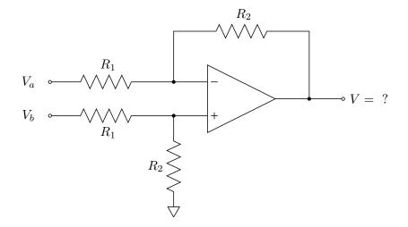
(a) Assuming that the op amp is ideal, use the op amp rules and conservation of energy and charge to derive the output potential V in terms of  $V_a$ ,  $V_b$ ,  $R_1$  and  $R_2$ .
