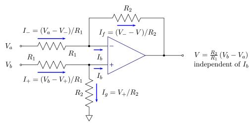
(b) Now suppose that both the inverting and noninverting inputs draw a small input bias current  $I_b$ . Using the same approach, derive an expression for V, and determine whether or not  $I_b$  appears in the output.
