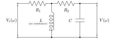
(a) Consider the circuit to be two consecutive filters with transmission functions  $A_1(\omega)$  and  $A_2(\omega)$ . Use physical reasoning and the concept of impedance to explain thoroughly the behavior of the each filter at low, intermediate and high frequencies. Clearly indicate where current is or is not flowing at low, intermediate and high frequencies. Pictures would useful.
