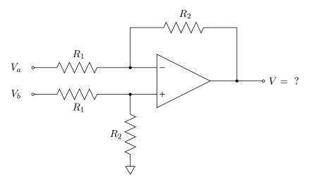
(a) Assuming that the op amp is ideal, use the op amp rules and conservation of energy and charge to derive the output potential V in terms of  $V_a$ ,  $V_b$ ,  $R_1$  and  $R_2$ .
