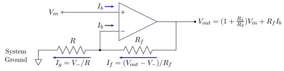
Begin with  $V_{out} = G(V_+ - V_-) = G(V_{in} - V_-)$ , so  $V_{in} \simeq V_-$ . Find the relation between  $V_-$  and  $V_{out}$  using  $I_f = I_b + I_g$ .
