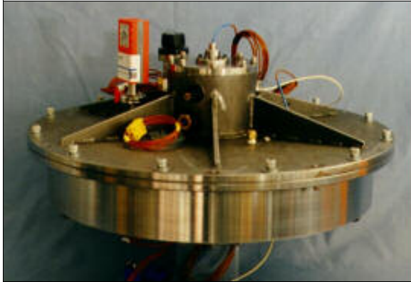
Figure 6 Attitude Control Energy Storage (ACES) System
