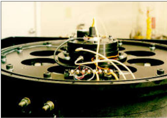
Figure 15 1.5 kW EMB Upper Instrumentation
