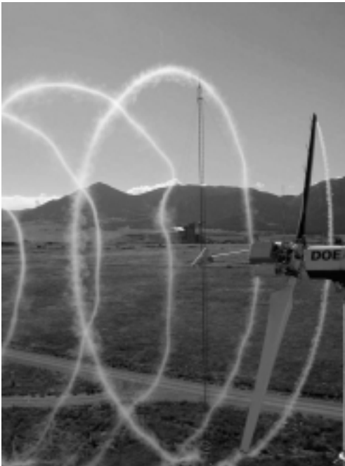
Figure 22.5 Aerodynamics research wind flow visualization study test at the National Wind Technology Center
