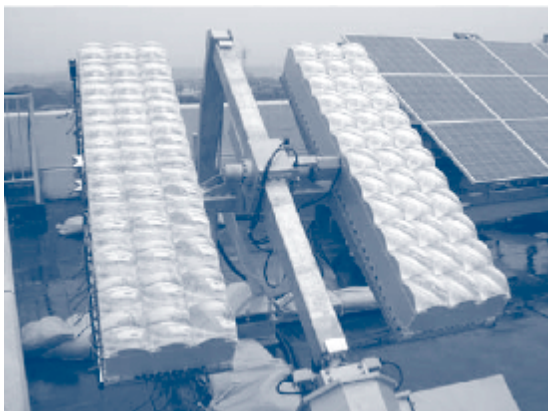
Figure 8. Daido Steel's Toyohashi 200-watt module is lightweight and uses high-efficiency multijunction cells—perfect for rooftop installation in population-dense places like Japan.
