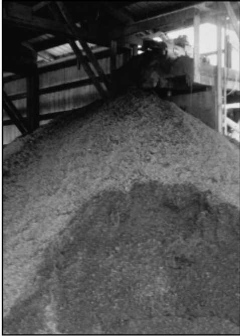
Fiber separated from the effluent collects below the separator and is stored before being sold or used. Leftover liquid continues on to the farm's storage lagoons.
