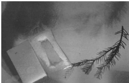
FIG. 5. Naturally buoyant analogous materials such as spruce or pine do not stimulate ice formation as effectively as porous polymers.
