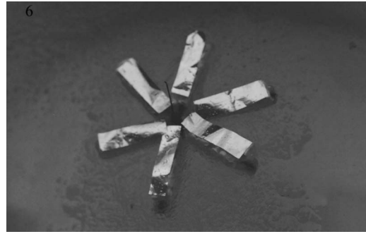
FIG. 6. Optimal construction keeps more thick ice near itself in warm weather.
