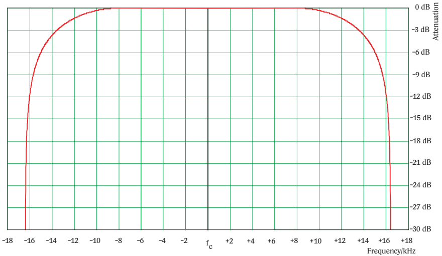
Fig. 6-24 Channel filter for IS-136 (NADC) systems
