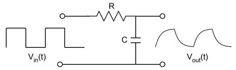
As the frequency of the applied square wave increases, the output waveform is diminished because there is insufficient time for the capacitor to charge to the applied voltage. Examining the expression for  $V_c(t)$  at times t small compared to  $\tau$ , we find
