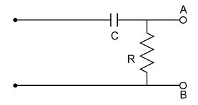
If we swap the positions of the resistor and capacitor, we have a *CR* circuit, where we measure the output voltage across the resistor. The Kirchoff loop analysis from above is still valid here, the only change being that  $V_{out} = V_R$ . Using the results from above, the output signal response to a square wave input is shown below. In this case, the input frequency is low and the circuit behaves as a differentiator.
