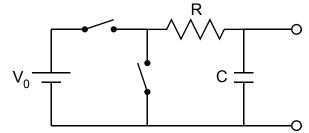
The behavior of this "*RC*" circuit can be analyzed in the time-domain by solving an appropriate differential equation with the appropriate boundary conditions. Begin with Kirchoff's Potential Law, which is a consequence of conservation of energy:
