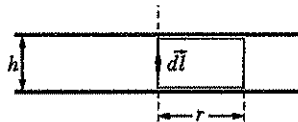
Figure 2: A loop for calculating the E -field, induced by the magnetic field.
