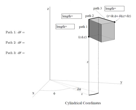
If all three coordinates are allowed to change simultaneously, by an infinitesimal amount, we could write this  $d\vec{r}$  for any path as:
