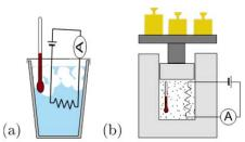
**FIGURE 1**: (a) Sketch of the ice calorimetry experiment performed on the first day of class. (b) Solution to a "name-the-experiment" activity in which students are asked to imagine an experiment measuring  $(\partial S/\partial T)_p$ . Students commonly point out the connection in the second name-the-experiment activity that this experiment is the same as they did in the first week of class.
