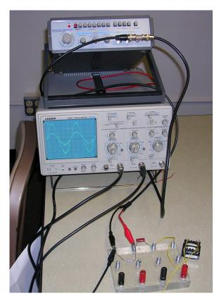
**Circuit breadboards**: plastic blocks with 12 springs glued into them. BNC "T", BNC (FG-scope), BNC-aligator (FG-circuit), scope probe (scope-resistor), wires.
