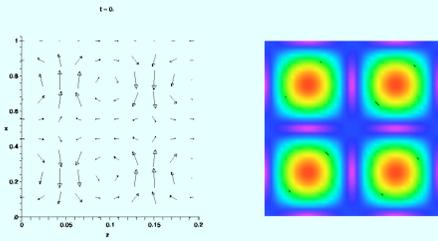
Student class work showing TE<sub>21</sub> mode in EM waveguide
