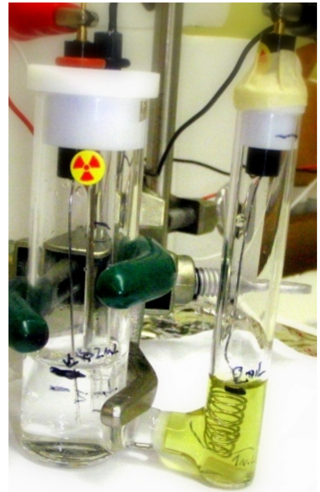
Hexavalent neptunium (15 mM) prepared electrolytically in 4M \text{HNO}_3 in H-cell with a Pt electrode (OSU, Nov 2009).
