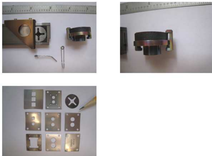
Fig. 6 Upper Left: a modified adjustable parallel used to clamp down a square substrate for scoring and cleaving. The wedge can be moved along the edge and serves as a straight edge to score the glass. A few millimeters of vertical clearance was built in so the straight edge never touches the film surface. Also shown in upper left are clips made from 10 gauge wire and spot welded to a 2-34 washer. These are used to clamp down the substrate to the heater block, providing firm pressure. At upper right, a \text{BaBiO}_3 target clamped to the target holder using a custom designed mini c-clamp allowing for easy target switch-out. A set screw allows a range of target heights to be accommodated. At lower left, several different style shadow masks. In the lower left image, the bottom far left piece is a substrate chuck for a 10 x 15 mm substrate. The chuck includes locating holes for a mask that fits over the substrate, giving perfect alignment. All of the other mask with small locating holes in their corners are used with this chuck. Some of the masks were laser-cut, but the chuck and the cross (upper right) were custom designed and fabricated at OSU.
