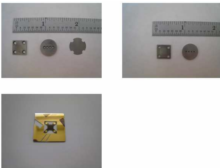
Fig. 8 (upper L image, from L to R) Deposition sides of masks used to deposit electrical contacts onto films patterned with the hall mask, an arbitrary four-point in-line pattern, and contacts on the surface of a pellet. The holes are countersunk to reduce shadowing. At above right, the reverse side of the masks. The square shaped mask was fabricated with a slight depression on the film side. In this way, the mask only touches the film at the site of the contacts and does not scrape the film center. This is important because film integrity is important for good electrical measurements. The bottom image is a \text{BaBiO}_3 film with gold PLD contacts deposited with this mask.
