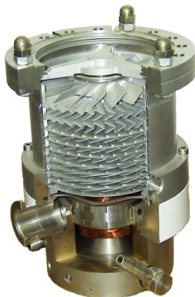
Figure 3.9: Photograph of a turbo pump with cut out showing the stator and rotor.
