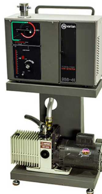
Figure 5.2: Varian model 938, Mass Spectrometer helium leak detector.
