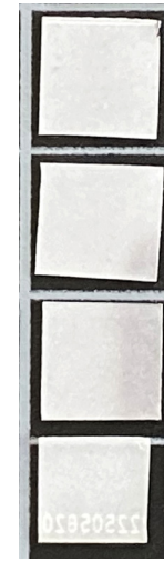
Figure 15. 5mm die cleaved from a 2" diameter sapphire wafer
