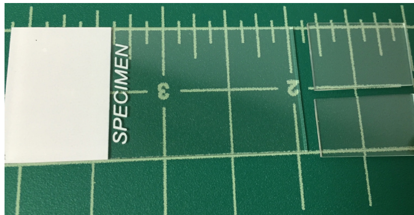
Figure 1. Scientific glass, 1 mm thick cut with the LatticeAx.
