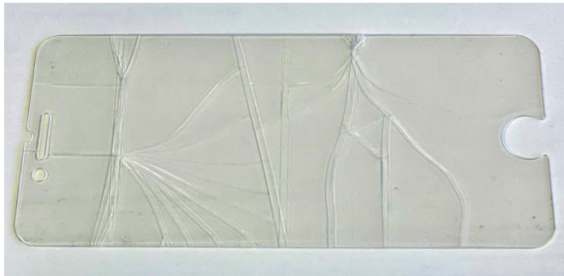
Figure 10. Cutting with a standard tungsten carbide scribing wheel resulted in a splintered sample.
