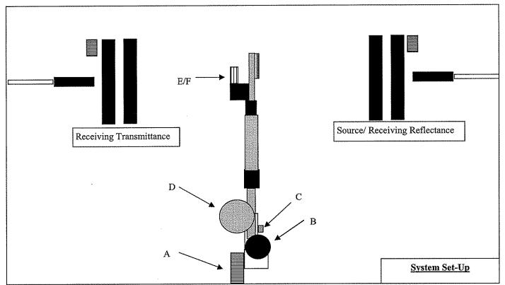
23. The next prompt will ask for the reflectance signal to be maximize. Raise the sample holder height so that the mirror is in the beams path. Use knobs E and F to angle the mirror so that the signal is maximized. Increase the integration time to 30,000. If the signal does not look like the screen shot, the system is out of alignment. Please get help aligning the system.
