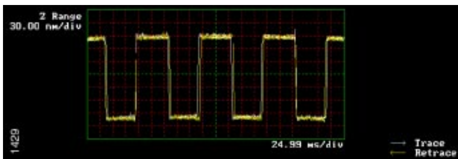
Figure 16.5 Scope Trace Demonstrating the High Frequency Noise that Occurs when the Integral Gain is Set Too High
