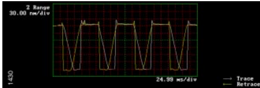
Figure 16.3 Scope Trace Demonstrating the Effect of the Setpoint Being Adjusted Too Close to the Free Air Amplitude During TappingMode AFM
