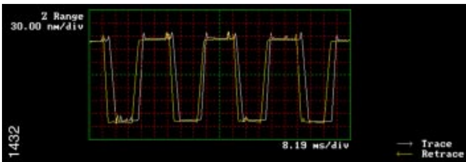
Figure 16.8 Scope Trace Demonstrating the Effect of Setting the Scan Rate Too High
