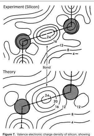
increased density in the space between nuclei associated with a covalent bond. Reprinted with permission from Reference 10. © 1989 Springer.
