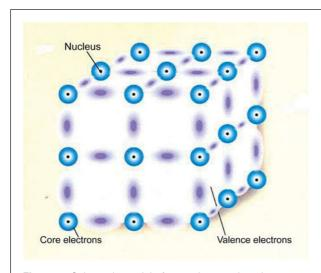
**Figure 4.** Schematic model of a covalent semiconductor showing the positions of atomic nuclei in black and the clouds of electrons forming bonds between them.
