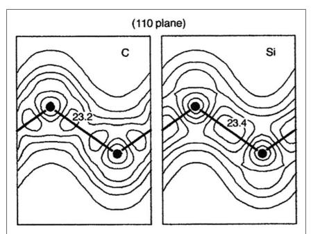
**Figure 8.** The effect of silicon's core *p* electrons is apparent in comparing the valence electronic charge density of solid carbon and silicon, where unlike silicon, the density of electrons in carbon has a double hump structure. Reprinted with permission from Reference 17. © 1973 AAAS.
