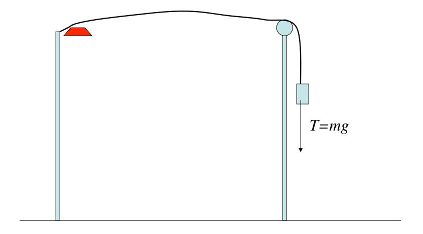
Generate standing waves in this system and measure values of  $\omega$  (or f) and k (or  $\lambda$ ).
