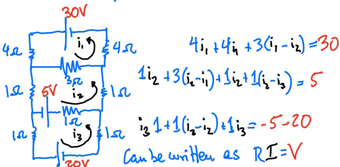
$$\text{where } \bar{L} = \begin{pmatrix} 1 & 0 & 0 \\ 0 & 1 & 0 \\ 0 & 0 & 1 \end{pmatrix} \quad R = \begin{pmatrix} 11 & -3 & 0 \\ -3 & 6 & -1 \\ 0 & -1 & 3 \end{pmatrix}$$
