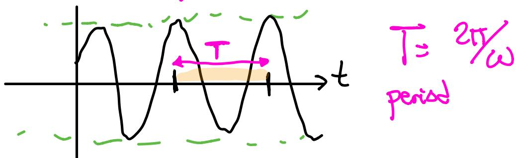
Ex) A mass weighing 2 lbs stretches a spring 6 inches. At  $t=0$  the mass is released 8 inches below equilibrium ( $u=0$ ) with an upward velocity of  $\frac{4}{3}$  ft/sec. There is no external forcing. Find the displacement as a function of time:
