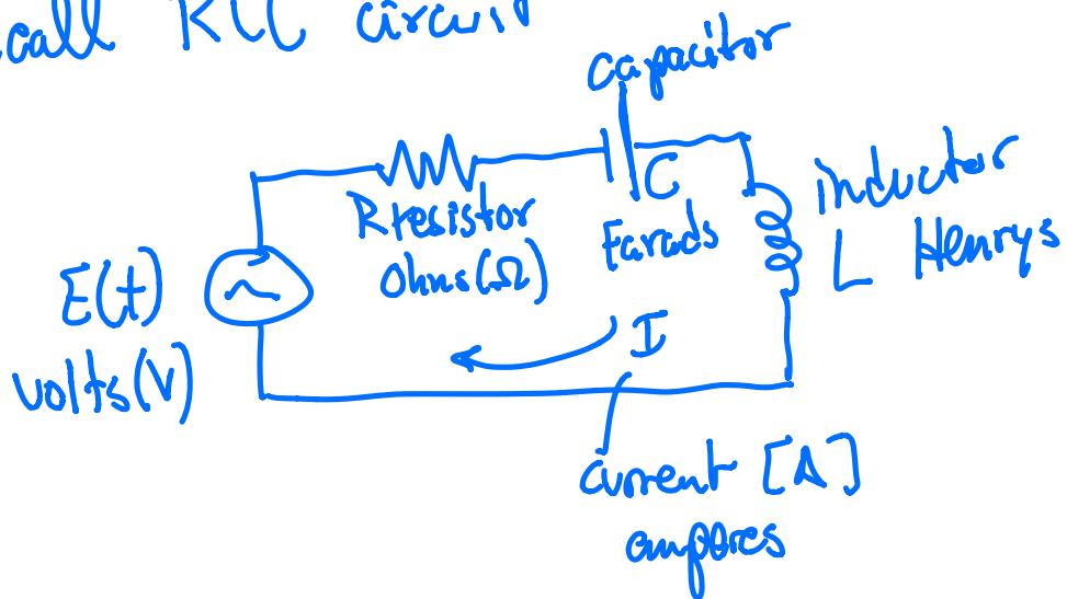
$$V_R = IR \quad \text{voltage drop in } R$$
