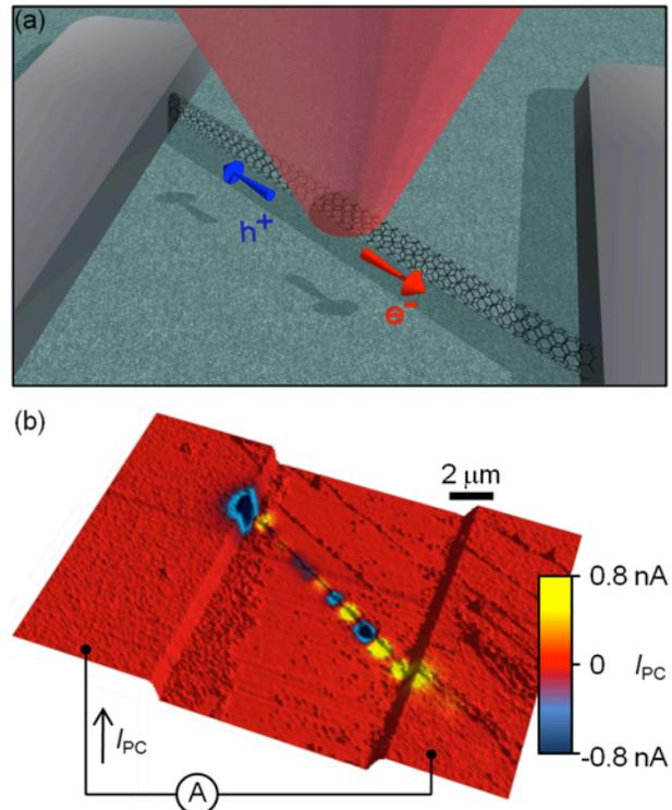
Fig. 1 SPCM Measurement Example. (a) Cartoon diagram of a scanning photocurrent measurement. (b) SPCM image from a CNT FET device taken at 632 nm, 800  $\mu$ W, and FWHM of approximately one micron. The photocurrent image has been superimposed onto an AFM height image of the device. The other nanotubes in the image do not make it across the electrode gap and show no photocurrent response.
