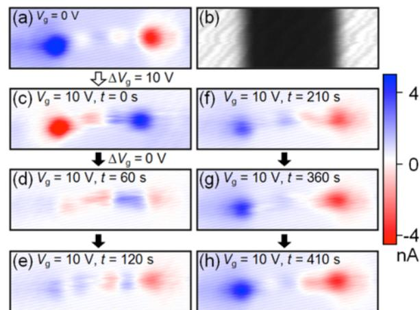
Fig. 5 Imaging CNT FET Hysteresis (a) SPCM image of device in Fig. 4 at  $V_g = 0$  V (b) Corresponding reflection image of device. (c) SPCM image taken immediately after sweeping  $V_g$  to 10 V. (d)-(h) Multiple SPCM images showing transient photocurrent behavior while  $V_g$  is held at 10 V. (d)  $t = 60$  seconds (e)  $t = 120$  seconds (f)  $t = 210$  seconds (g)  $t = 360$  seconds (h)  $t = 410$  seconds.
