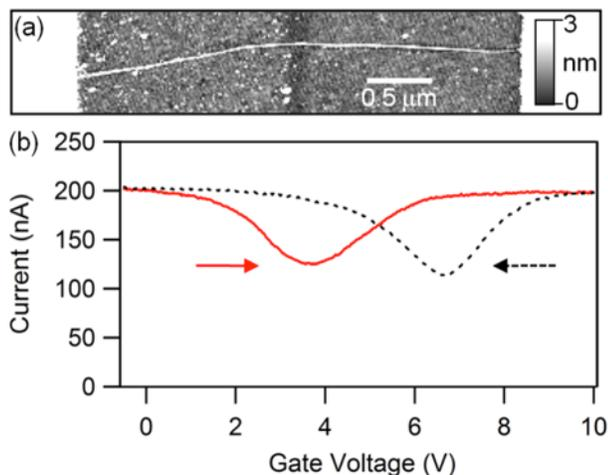
Fig. 4 Ambipolar CNT FET (a) AFM Height image of CNT on SiO<sub>2</sub> crossing electrode gap. Scale bar is 0.5 μm. (b) Transistor curve of device. The solid (dashed) curve is an increasing (decreasing)  $V_g$  sweep.  $V_{sd} = 25$  mV,  $dV_g/dt = 0.5$  V/s.
