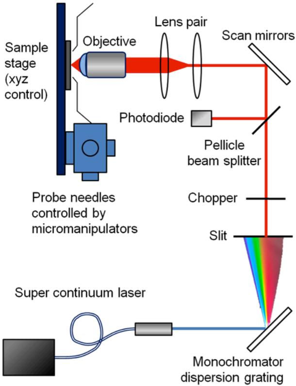
Fig. 2 Schematic Diagram of Scanning Photocurrent Microscope.
