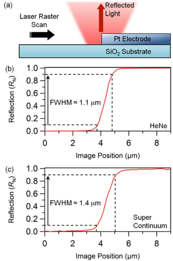
Fig. 3 Spot Size Characterization from Reflection Images. (a) Cartoon diagram of laser spot halfway onto a metal electrode corresponding to  $R_N = 0.5$ . (b)  $R_N$  of electrode edge from HeNe laser. (c)  $R_N$  of electrode edge from super continuum laser with monochromator output set to 632.8 nm and 1 nm bandwidth.
