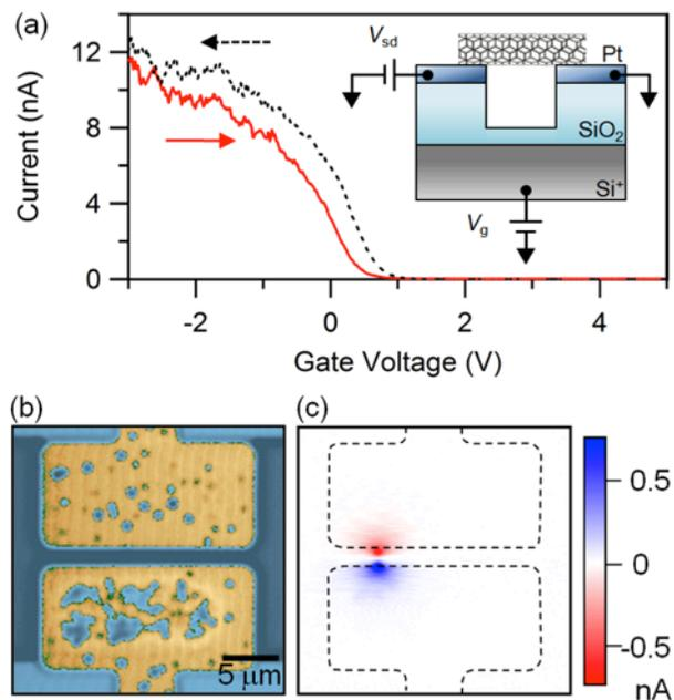
Fig. 6 Suspended CNT FET with Large Band Gap (a) Transistor curve of device.  $V_{sd} = 25$  mV,  $dV_g/dt = 0.5$  V/s. Inset shows device geometry (b) Reflection image of device. (c) Short circuit photocurrent image of device taken with lock-in amplifier.
