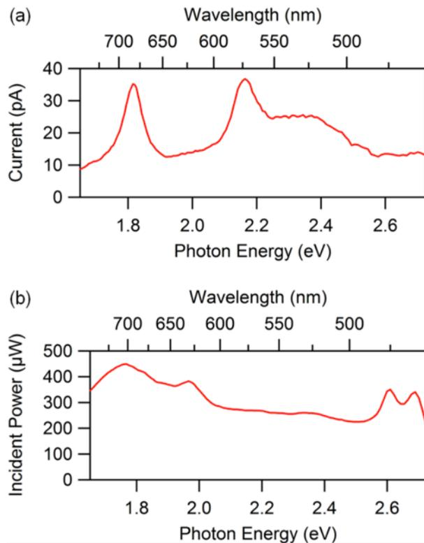
Fig. 7 Spectral Dependence of Suspended CNT FET. (a) Measured change in current as photon energy is varied. (b) Power incident to sample as a function of photon energy.
