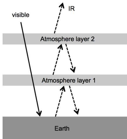
The Figure shows a two-layer model, similar to the one-layer model we did in class. Both atmospheric layers are transparent to visible light. The atmospheric layers absorb, thermalize and re-emit infrared radiation.
