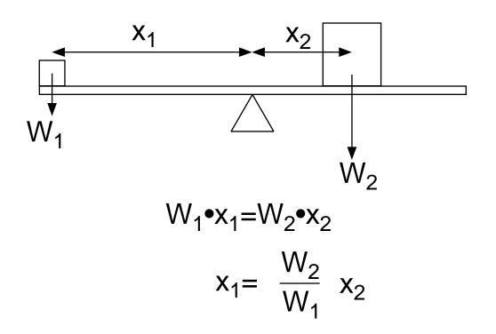
The weights must be positioned to keep the center of mass directly above the pivot point (or fulcrum)
