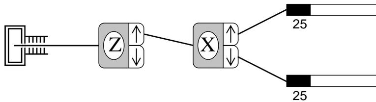
An experiment for successive measurement of spin projections.
