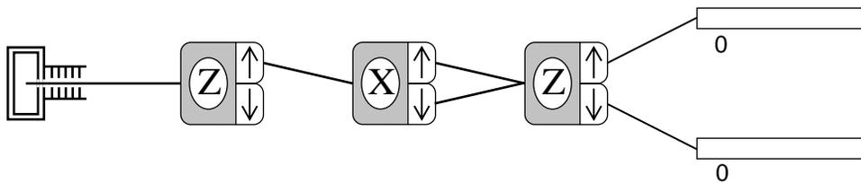
An interference experiment with spin  $1/2$  particles.
