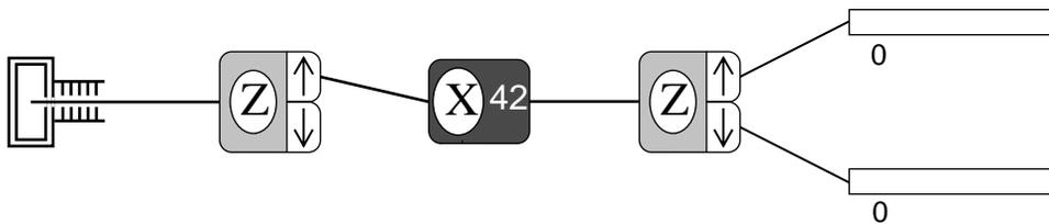
An experiment to study spin  $1/2$  particles in a magnetic field.
