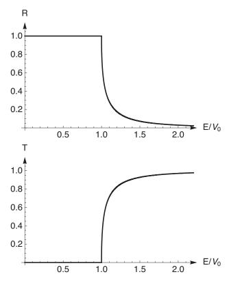
The reflection is unity until the energy exceeds the step height, after which the reflection decreases monotonically. In the limit of large energy,  $T \rightarrow 1$ , as you might expect because the step becomes insignificant.
