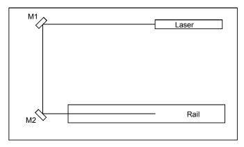
The U geometry is defined by the two mirrors labeled M1 and M2 in the diagram. The goal of this experiment is to ensure that the laser beam (i.e. the optical axis) is parallel to the table top and aligned above the center of the rail. Mount M2 on the optical table and position it close to the beginning of the optical rail such that the center of the mirror is above the center line of the rail and is at a height greater than 14.5 cm above the table (**this height will ensure that**
