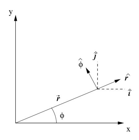
$$\frac{d^2\vec{r}}{dt^2} \equiv \ddot{\vec{r}} = \vec{a} = (\ddot{r} - r\dot{\phi}^2)\hat{r} + (r\ddot{\phi} + 2\dot{r}\dot{\phi})\hat{\phi}$$
