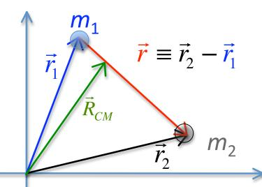
Relative motion obeys a single-particle equation. Fictitious particle, mass  $\mu$  moving in a central force field. Vector r measures RELATIVE displacement; we have to "undo" to get actual motion of each of particles 1 and 2. Often m1>>m2.
