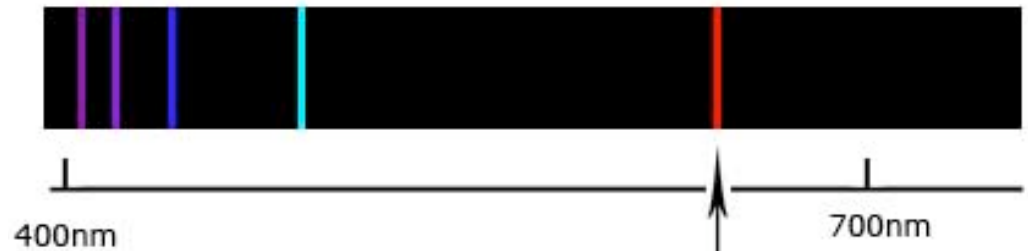
Hydrogen Emission Spectrum
