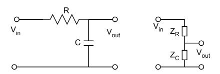
The behavior of this RC circuit can be analyzed by treating it as the voltage divider shown at right. The output voltage is then
