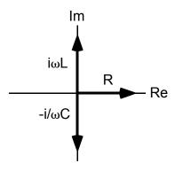
These phasors are useful because the voltage across each circuit element is related to the current through the equation V = IZ. For a series circuit where the same current flows through each element, the voltages across each element are proportional to the impedance across that element.
