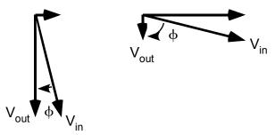
The diagrams demonstrate that at  $\omega \ll \omega_c$ :  $V_{out} \simeq V_{in}$  and  $\phi \to 0$  and at  $\omega \gg \omega_c$ :  $V_{out} \to 0$  and  $\phi \to -90^\circ$ .
