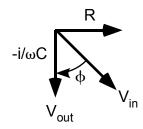
$$\frac{V_{out}}{V_{in}} = \frac{Z_C}{Z_C + Z_R} = \frac{-i/\omega C}{-i/\omega C + R}$$
