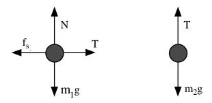
Since there is no motion of the system, all accelerations are zero and the equations of motion are:
