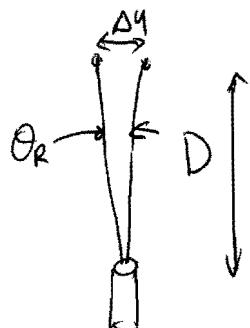
$$\Delta y = D \theta_R = (380,000 \text{ km})(1.32 \times 10^{-7} \text{ rad}) \\ = 50 \text{ m}$$
