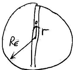
By the 2nd shell theorem, all the mass beyond radius  $r$  does not contribute to the gravitational force at  $r$ .
