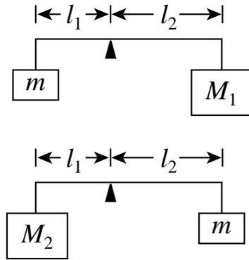
A rod of negligible mass is pivoted at a point that is off-center, so that length  $\ell_1$  is different from length  $\ell_2$ . The figures above show two cases in which masses are suspended from the ends of the rod. In each case the unknown mass  $m$  is balanced by a known mass,  $M_1$  or  $M_2$ , so that the rod remains horizontal. What is the value of  $m$  in terms of the known masses?
