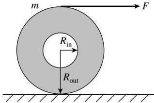
What must the magnitude of the force of friction be if the cylinder is to roll without slipping?
