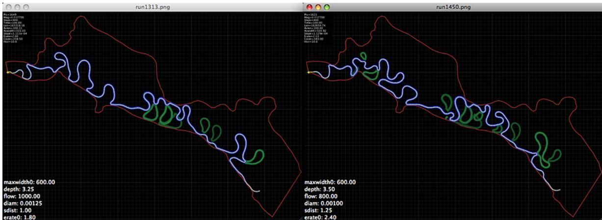
Figure 35: Two rivers within 0.1 standard deviations of the average final length and erosion rate.
