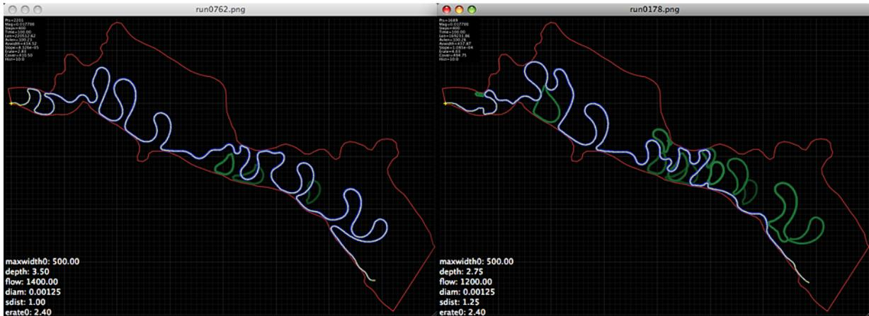
Figure 33: The longest river (left) and the river with the greatest coverage area (right) limited to simulations with an initial erosion rate of 2.4 ha/yr/km.
