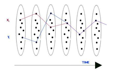
Coupling time:  $T_{coupling} = \min\{t: X_t = Y_t\}$
