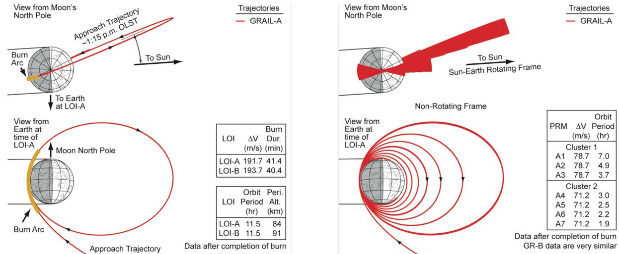
**Figure 11. LOI and OPR Phase Trajectories**
