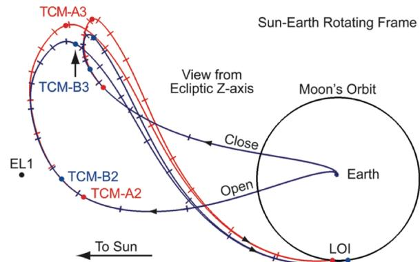
**Figure 10. Trans-Lunar Cruise Phase Trajectories**
