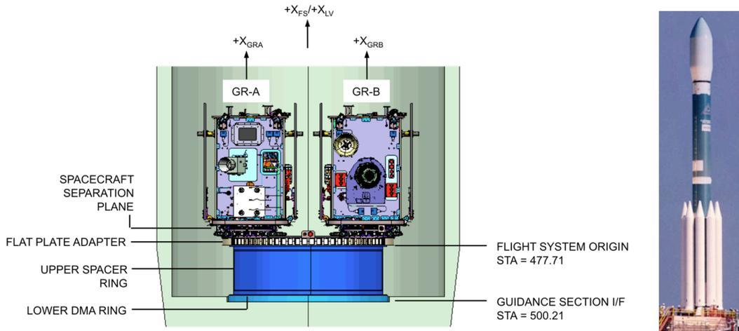
**Figure 5. GRAIL Launch Configuration**
