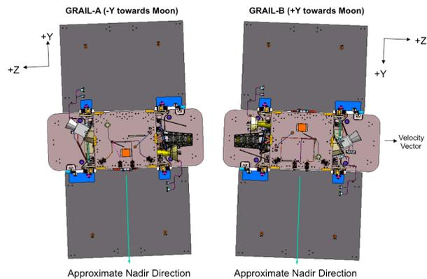
**Figure 18. Orbiter-Point Attitude During the Science Phase**
