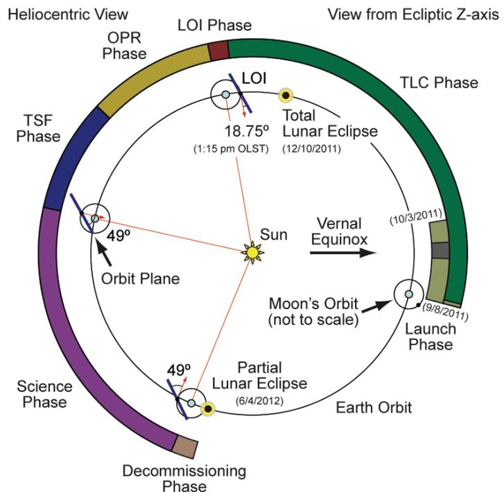
**Figure 2. Heliocentric View of GRAIL Mission**
