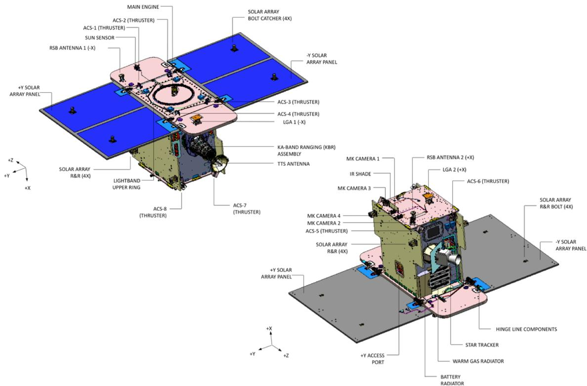
**Figure 4. GRAIL Orbiter Configuration**
