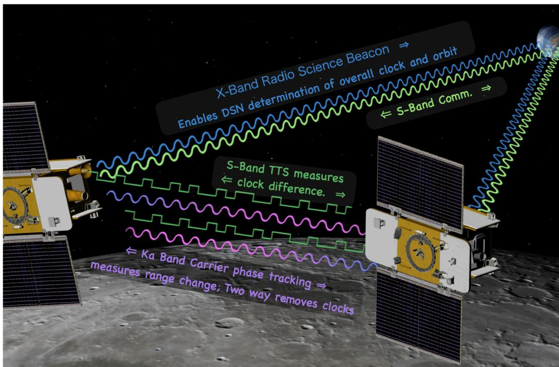
Figure 1. GRAIL Gravity Measurement
