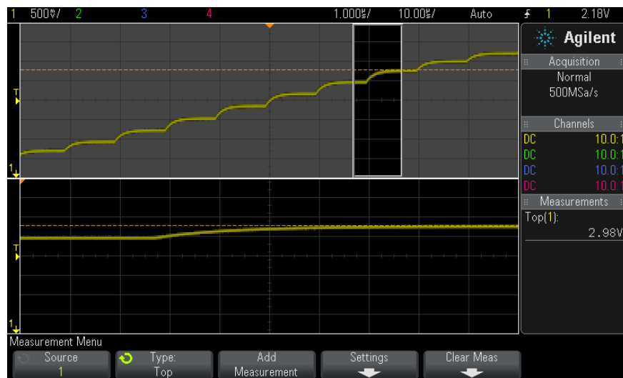
Figure 33 Isolating area for Top measurement
