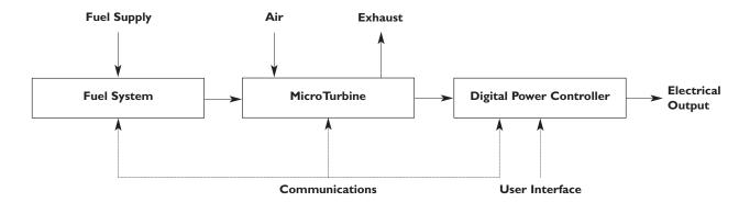
The Capstone Model 330 MicroTurbine system is a compact, low emission, power generator providing electrical power up to 30 kW. Solid-state power electronics allow grid-connect operation; stand-alone battery support and automatic grid/stand-alone switching are available options.
